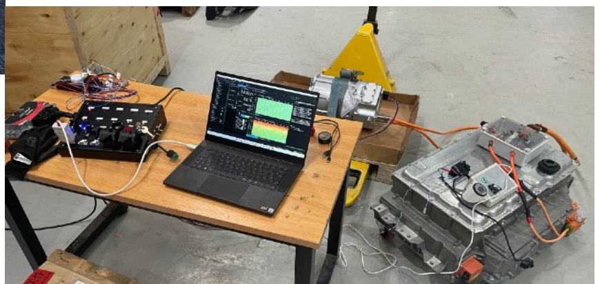
TESTING MOTOR AND VCU ON BENCH SETUP
