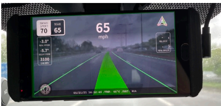
AUTOPILOT ENGAGED, SHOWING LANES AND PATH PLAN
