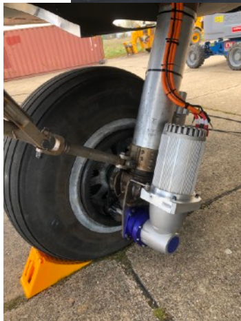
ONE MOTOR ON EACH FRONT WHEEL
